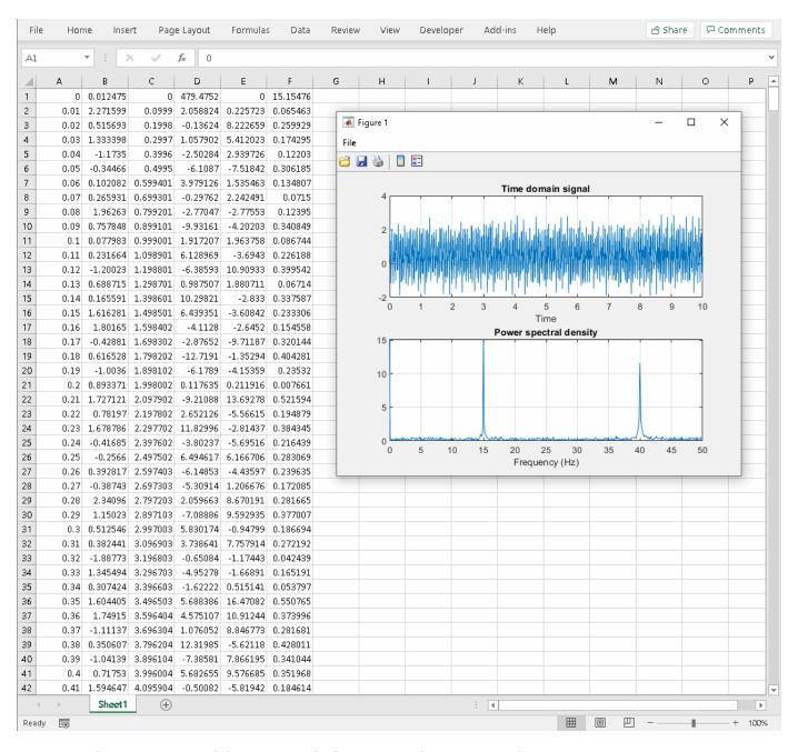
The power spectral density reveals the two signals at 15 Hz and 40 Hz.
